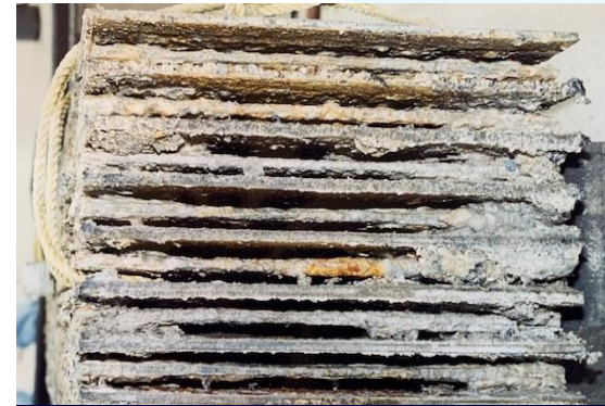
waterStrider Discovery: Lithium Scale on Water Treatment Cell
